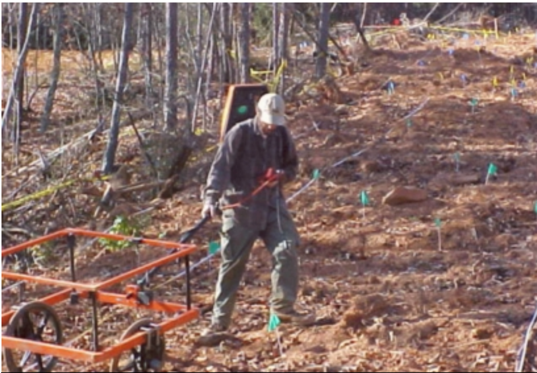
Photograph #16: NAEVA Geophysicist performing anomaly reacquisition with EM61 on Grid F08N
