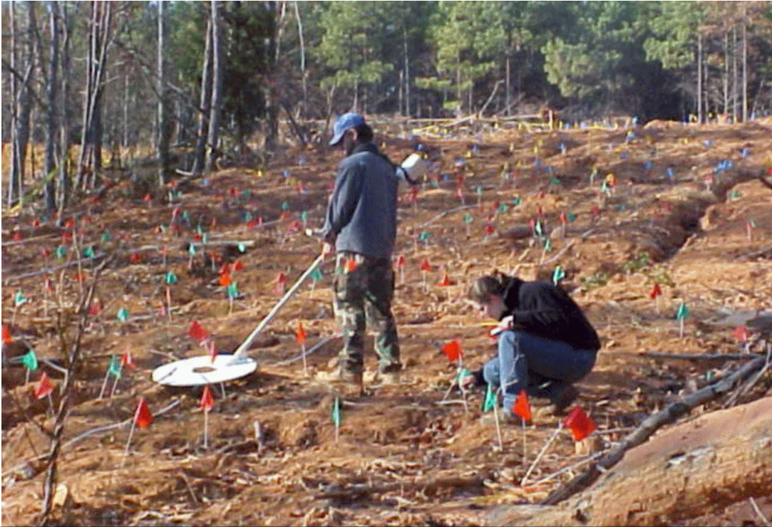
Photograph #17: NAEVA Geophysicists performing reacquisition with GEM3 on Grid F09N
